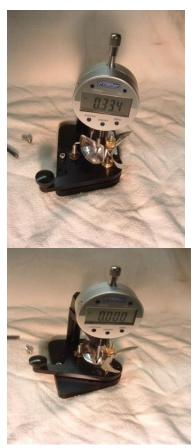
RESET zero point and then lift stem at top of indicator and reset swing plate. Gently drop tip back onto blades surface then travel back down from above as is typical. (This places stop point of swing plate at blades leading edge)
