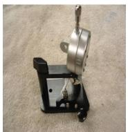
\* Distance value on indicator is now multiplied X20 when 2 screws are in place & X10 if only one.
