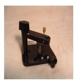
\*\* The amount of swing angle is halved when 2 screws are in place which allows less distance to be covered on blades face making tip cupping or specific areas of blade much easier to figure.
