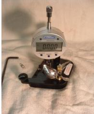
Turn on indicator, now wiggle stuff around making sure all is snug (Indicator reading will bounce if some things loose) One satisfied your ready to take a measurement and TIP of indicator is where you wish to measure from RESET the Zero on indicator. Next simply rotate the swing plate allowing tip of measuring stem fall down along face of blade until swing plate stops against the second screw..... Simple huh.
