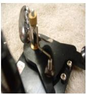
Your next blade is in the EXACT same place you were before. (Note: Wire stop is light duty and not strong enough to hold against hub rotation at arbor, Nut on back side of props hub must be firmly tightened)
