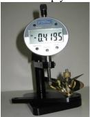
Start out with a simple reading by having both stop screws in place. Position a prop blade on arbor post adjusting stop wire so tip on indicator rests inward of outer most tip @ 1/4" or more while swing plate is full forward flush with base plate. Tighten Wire stop, Riser wing nut and
