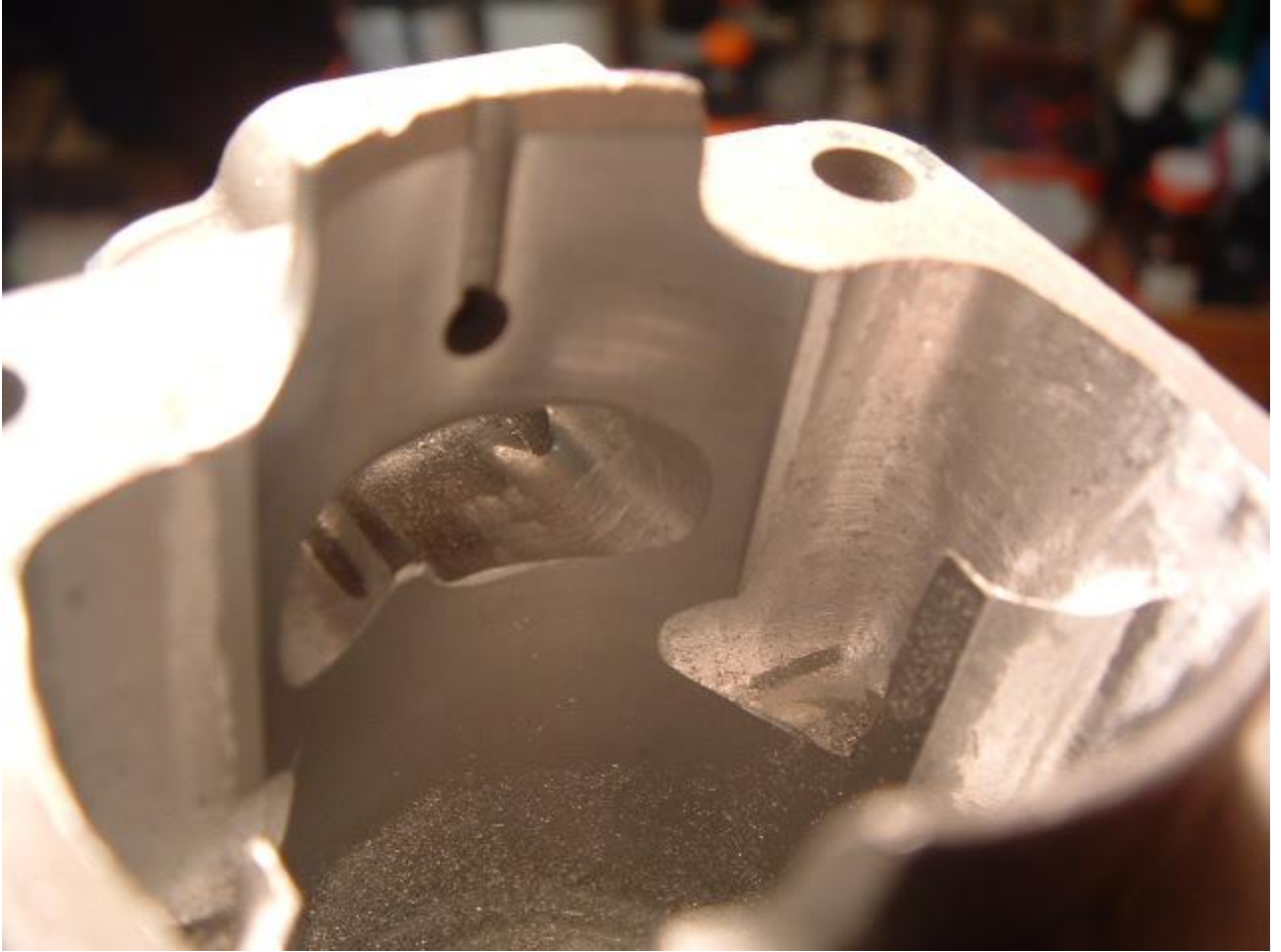
The other side of intake port, just widened. (cutter #2)
