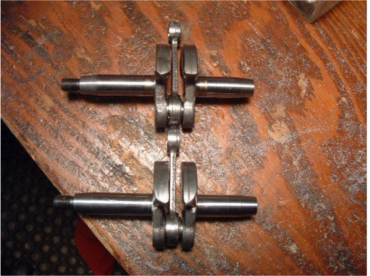
Crankshaft Turbo mod, shown with a stock one. (1" belt sander)
