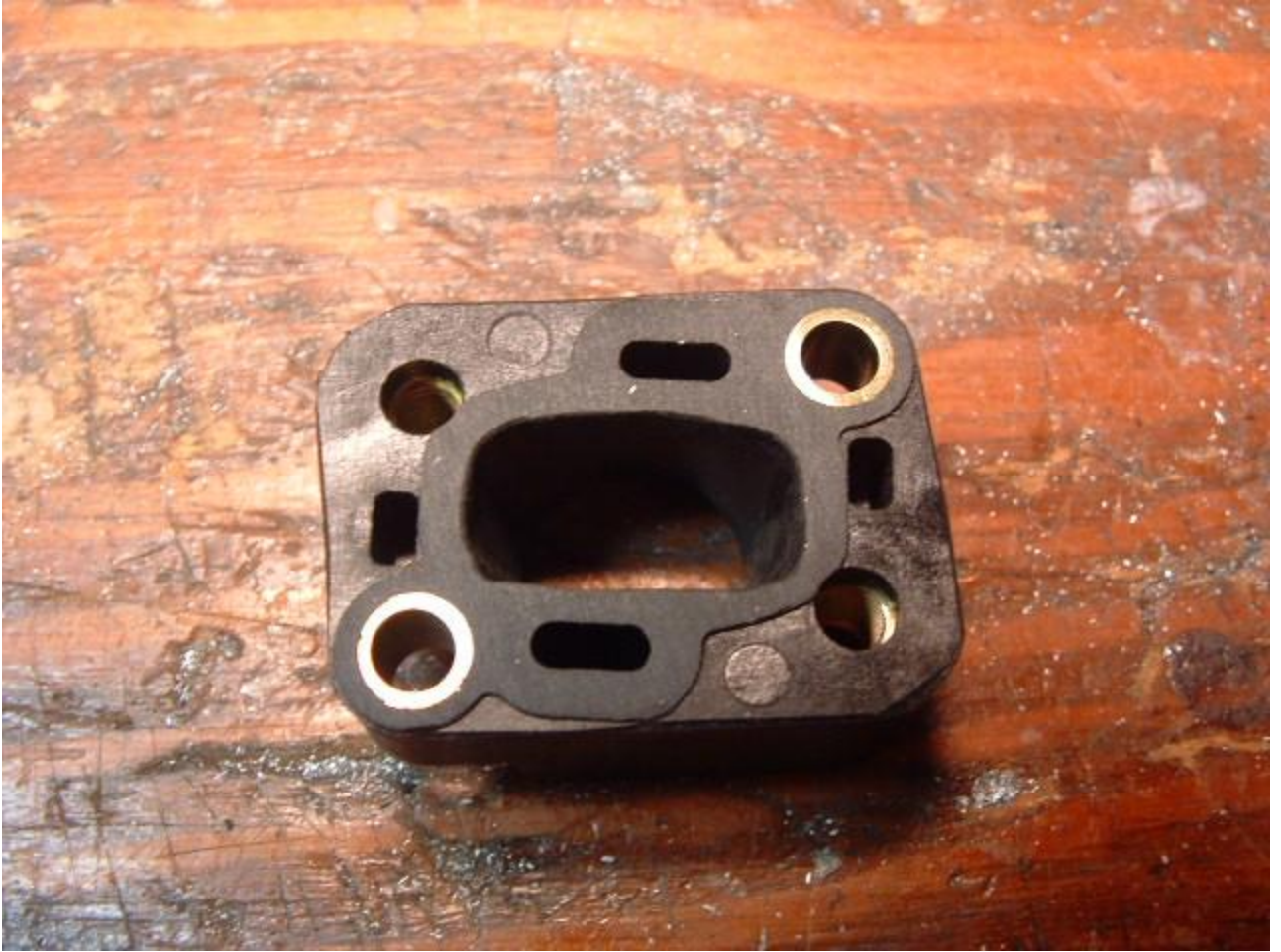
The intake manifold opened up to match cylinder & carburetor end opened up to .625" diameter. (cutter #2)
