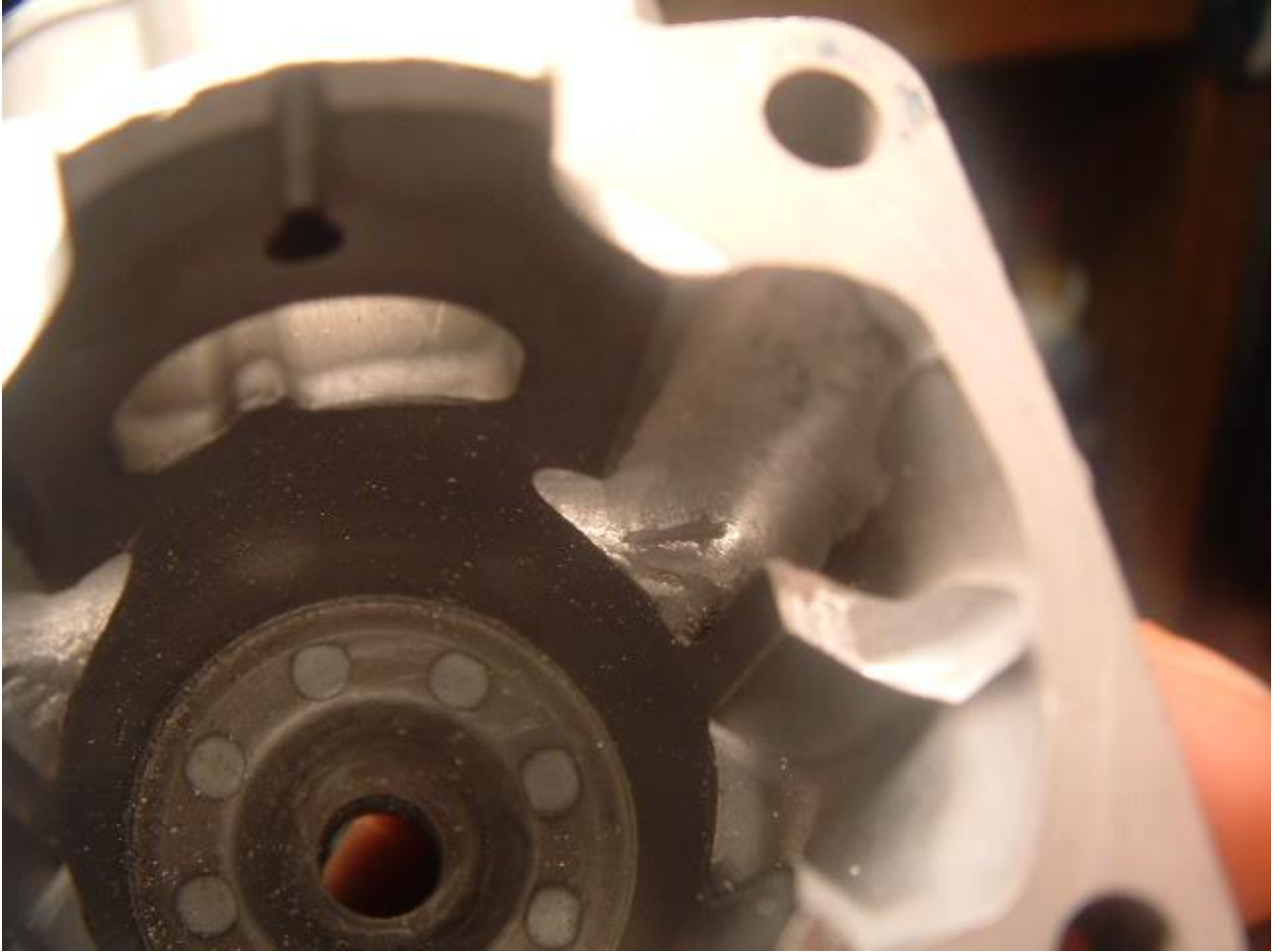
This photo the intake side transfer runner all cut and blended into eyebrow. (blended in with cutter #4)
