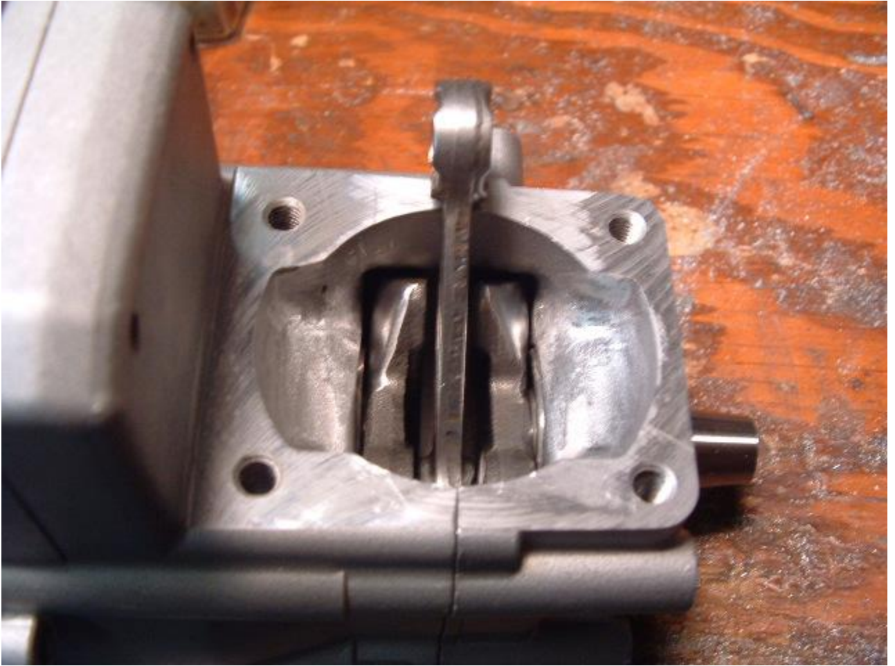
How cases look with crank installed. (view is crank position 90 degrees BBDC)
