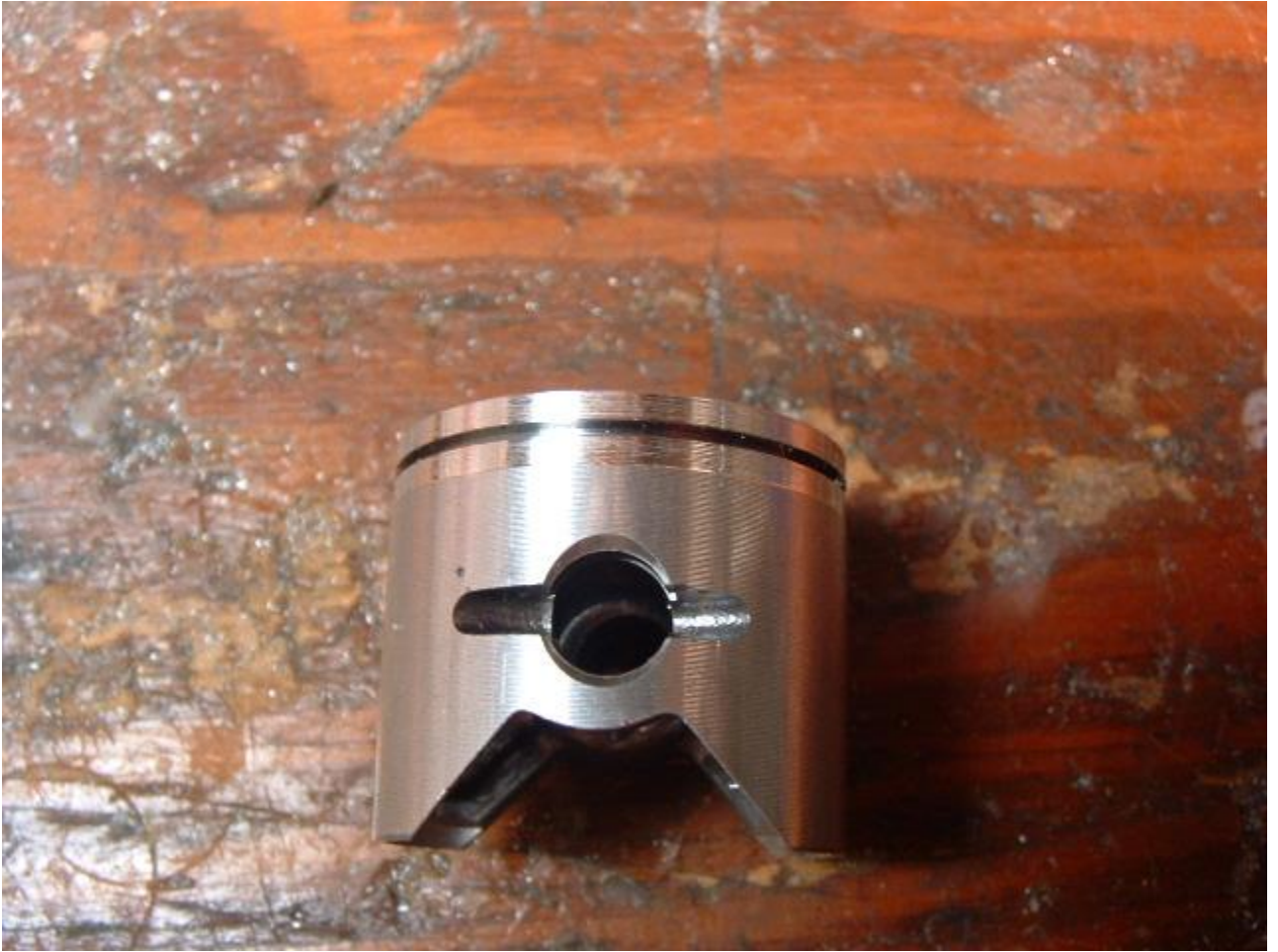
.002" cut made on top of piston (Total of .004" of diameter)
