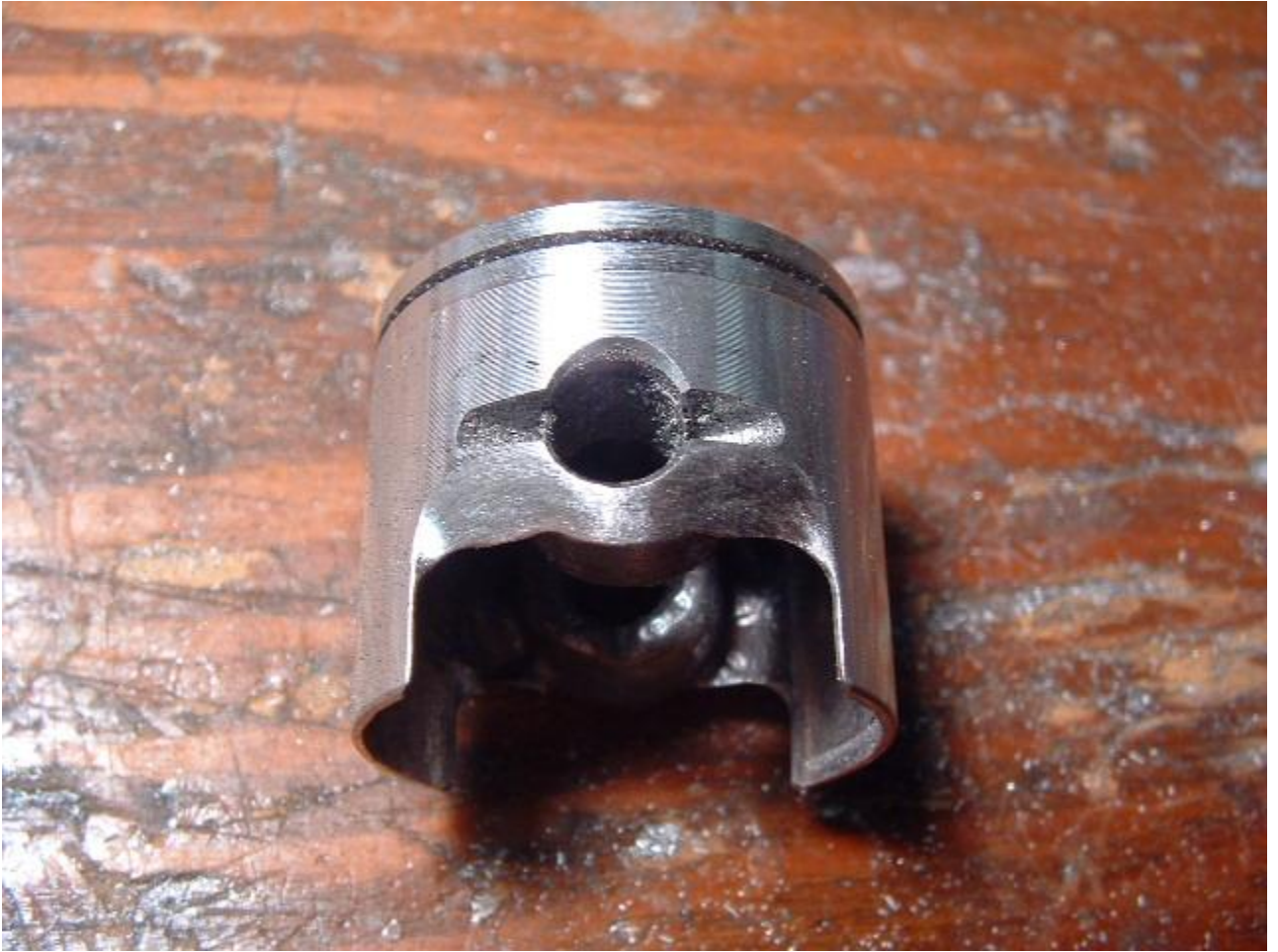
Area outside of pin boss area cut to force flow outward into transfer passages. (cutter #2)
