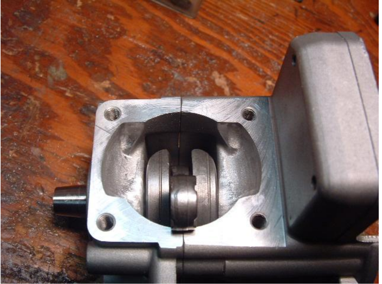
Crank position just BBDC (Note : factory ramps in cases left there & for GOOD reason) ramps direct charge up Ex side transfer edge.
