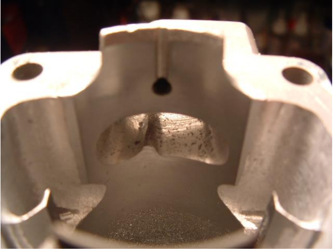
View once intake port was cleaned up and finished. (cutter #2 & #4)
