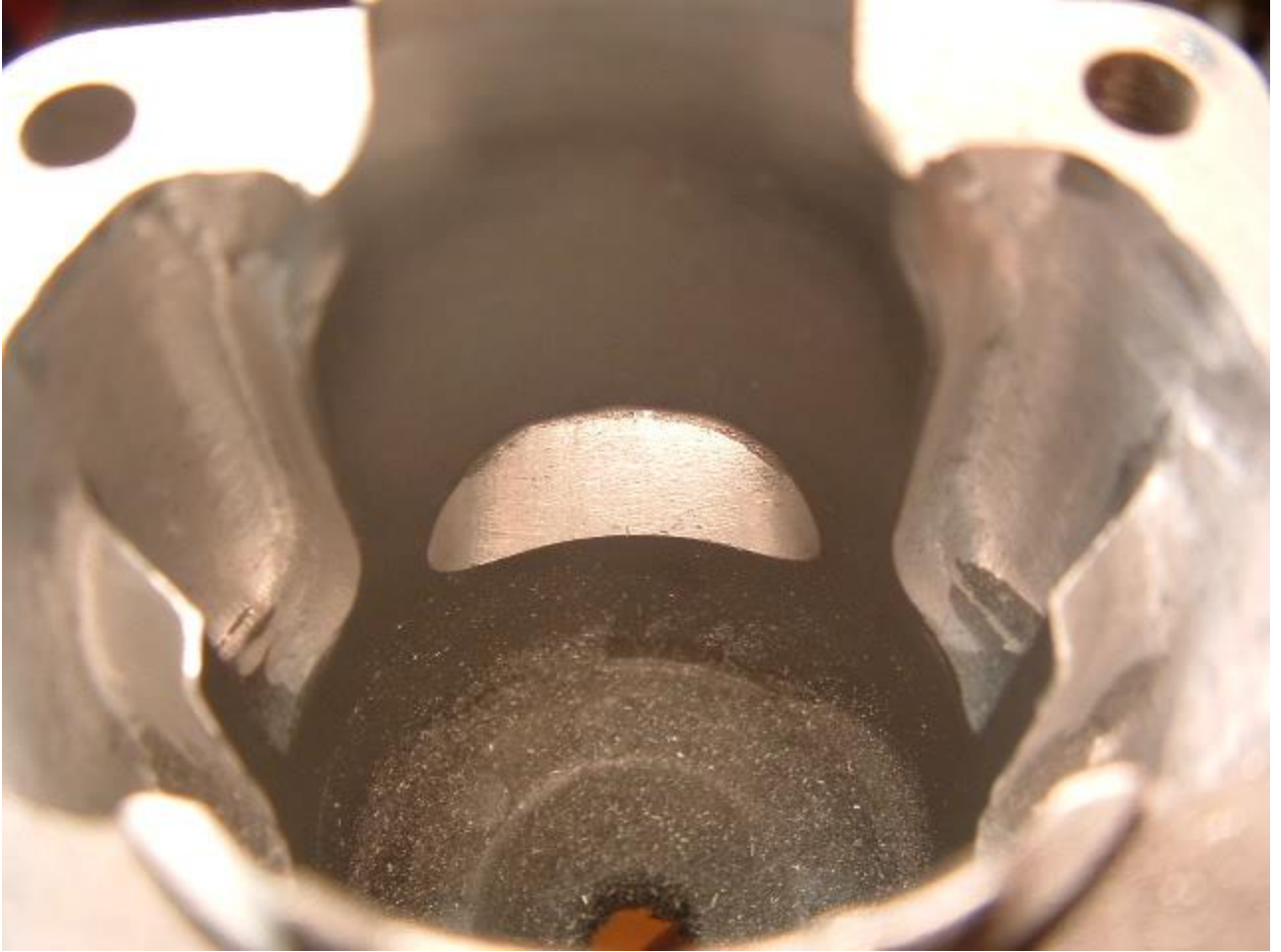
Stock exhaust port & once modified to @178 degrees. (cutter #2)
