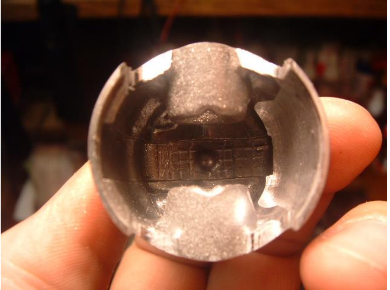
V shape cut out to increase area, also 1/2 of lightening process removing material that would support a second ring. Other side not done yet. (cutter #2)
